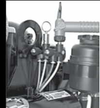
Air Actuated Single-Point Drain on FWC or SeaCore models
