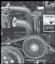
Single-Point Drain on Alpha drive models
